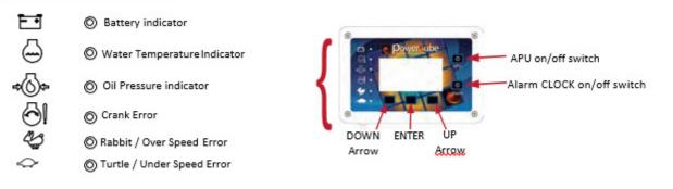
Battery Indicator: A voltage drop at or below 12 volts during cranking or normal operations.
