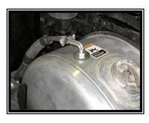
system and moving components. Fuel lines must be run along the frame side rails or under carriage. IMPORTANT: Never run fuel lines inside the cab.
